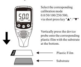
Note:It is important that measuring the standard film thickness with corresponding film calibration status. So when you find that you run this instrument calibration status with a mistake and some errors information shows on the display, we recommend to do the restore of factory operate.
